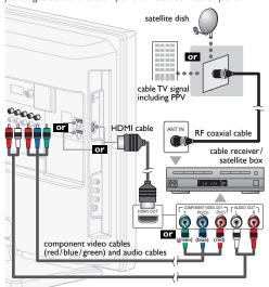
You can also connect this unit to the cable receiver or satellite box other than the HDMI or the Component Video output jacks or Composite Video output jack (IIIII) p.24, 25) because they might have different output jacks.
